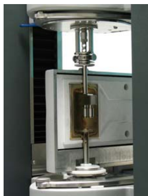
Fig. 1: SER tool integrated in Controlled Test Chamber
